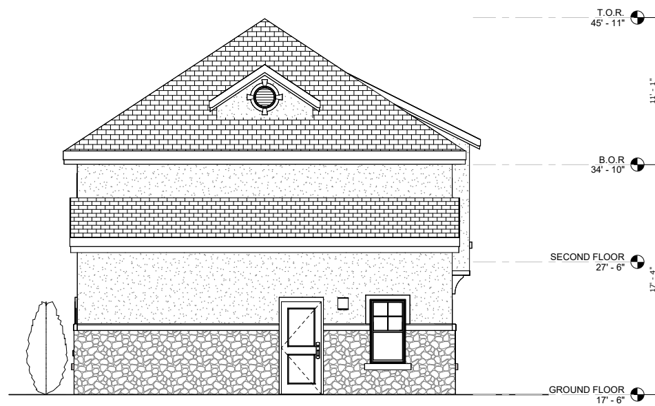
② RIGHT FACING ELEVATION 1/4" = 1'-0"
