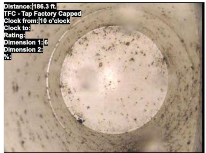
Distance: 186.3 ft. TFC - Tap Factory Capped Clock from: 10 o'clock Clock to: Rating: Dimension 1: 6 Dimension 2: %: Photo: 1-215-1-212-20221025-091723-093424.JPG At: 186.343 ft. TFC - Tap Factory Capped 10/. Joint: No
