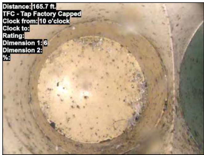
Distance: 165.7 ft. TFC - Tap Factory Capped Clock from: 10 o'clock Clock to: Rating: Dimension 1: 6 Dimension 2: %: Photo: 1-215-1-212-20221025-091723-093331.JPG At: 165.727 ft. TFC - Tap Factory Capped 10/. Joint: No
